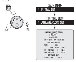
**2** Turn the J-dial, select the MODE under <DAYLIGHT SAVING>, and turn the S-dial clockwise.
